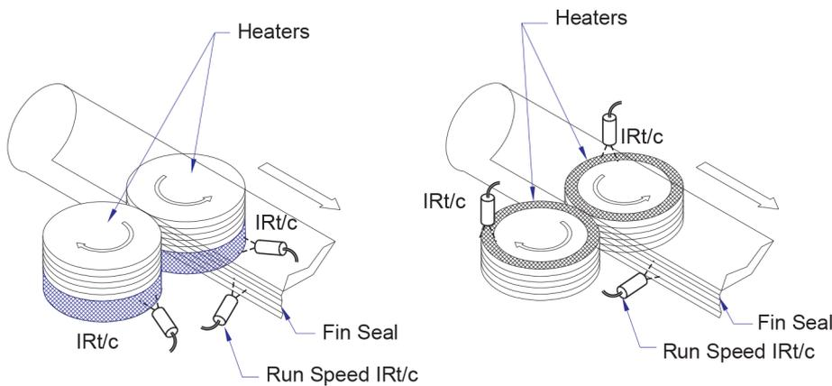
There are at least two choices for a reliable infrared target surface that meet the needs of the packaging industry (able to withstand repeated daily cleanings, durable to provide years of service):
