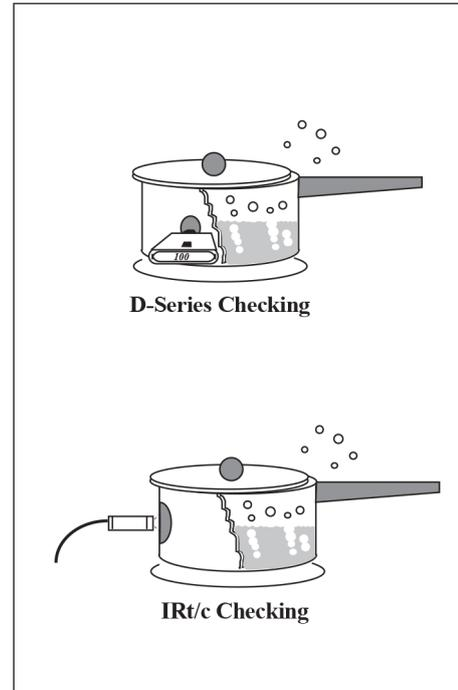
The reading should be within  $\pm 2\%$  of the actual boiling point (for example  $\pm 2^\circ\text{C}$  for  $100^\circ\text{C}$  boiling point). If the reading is not within these limits, the instrument has a failed component and should be returned to Exergen for repair. Please call for an RMA number prior to shipment. For the IRt/c refer to *Tech Note No. 73* for specifications.
