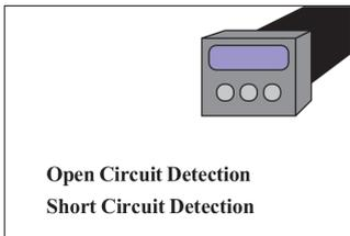
As in all thermocouple installations, a primary protection recommended is open circuit detection, which will alert if wires are
