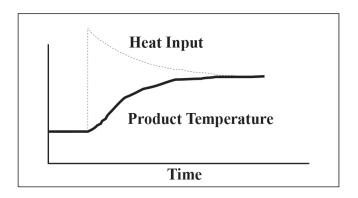
Microscanner D-Series (see Tech Note #1), initiate the self-tuning cycle of the controller and check to see that the control is stable and accurate. If it will not self tune properly, manually adjust the control coefficients to achieve stable control. Because the product temperature is likely to change temperature more slowly than the original sensor, start with slowly increasing the "D" of the PID coefficients.
